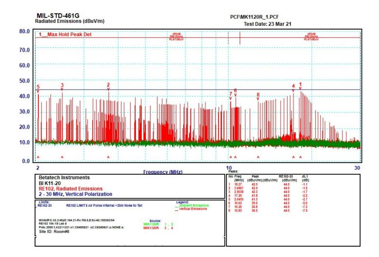
When the LED light is disconnected from the power (+) terminal, effectively removing the LED light from the test setup while still keeping the wire attached to the KEY terminal of the BI K11-20 board, we see a significant reduction of the broadband spike occurrences. The remaining spikes, when listened to, correspond to the relay (dit and dash) on-off of the robot:
